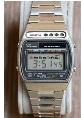
Seiko LCD Solar Alarm Chronograph A156-5000, 1978: Seiko's first solar-powered watch
